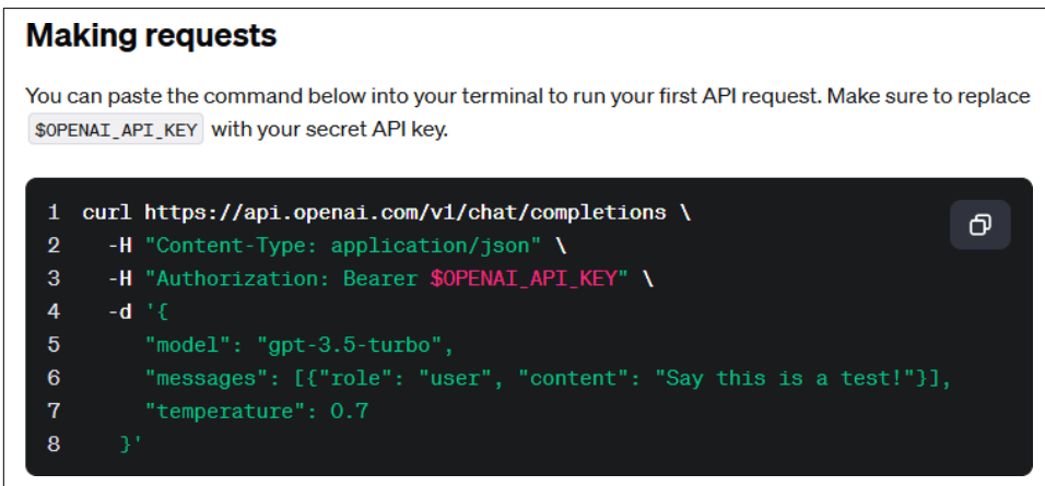
Figure 7-14. Create completion page
